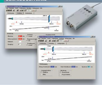
With the 3RX4000 PC interface and the SONPROG software, you can easily adapt the F65 and F260 ultrasonic sensors to the requirements of your specific application.
